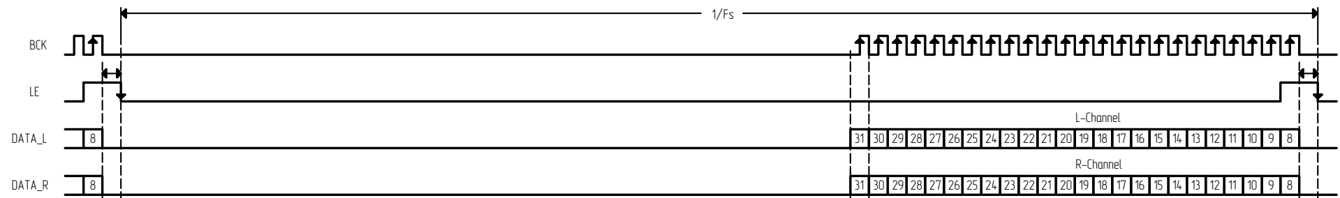
NOS DAC Data format. FULL SPEED & STOP BITCLOCK. Audio data word = 24 bit
