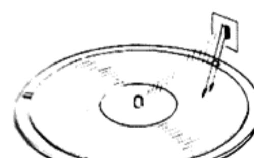
the tonearm lowers to the same point if a 17 cm record were on the platter, since only the inner holes are covered. To play a 25 cm record, move the tonearm over the record and lower the tonearm to the lead-in groove by pressing the  $\nabla/\underline{\nabla}$  button then press the START/STOP button.
