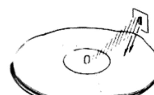
if the record is badly warped, a beam may pass through the holes to the detector and cause malfunction of the auto record size selection.
