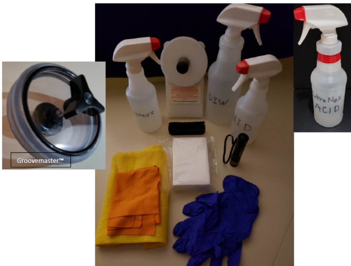
Figure 12 - Step 1: Assemble Cleaning Process Solutions and Materials
