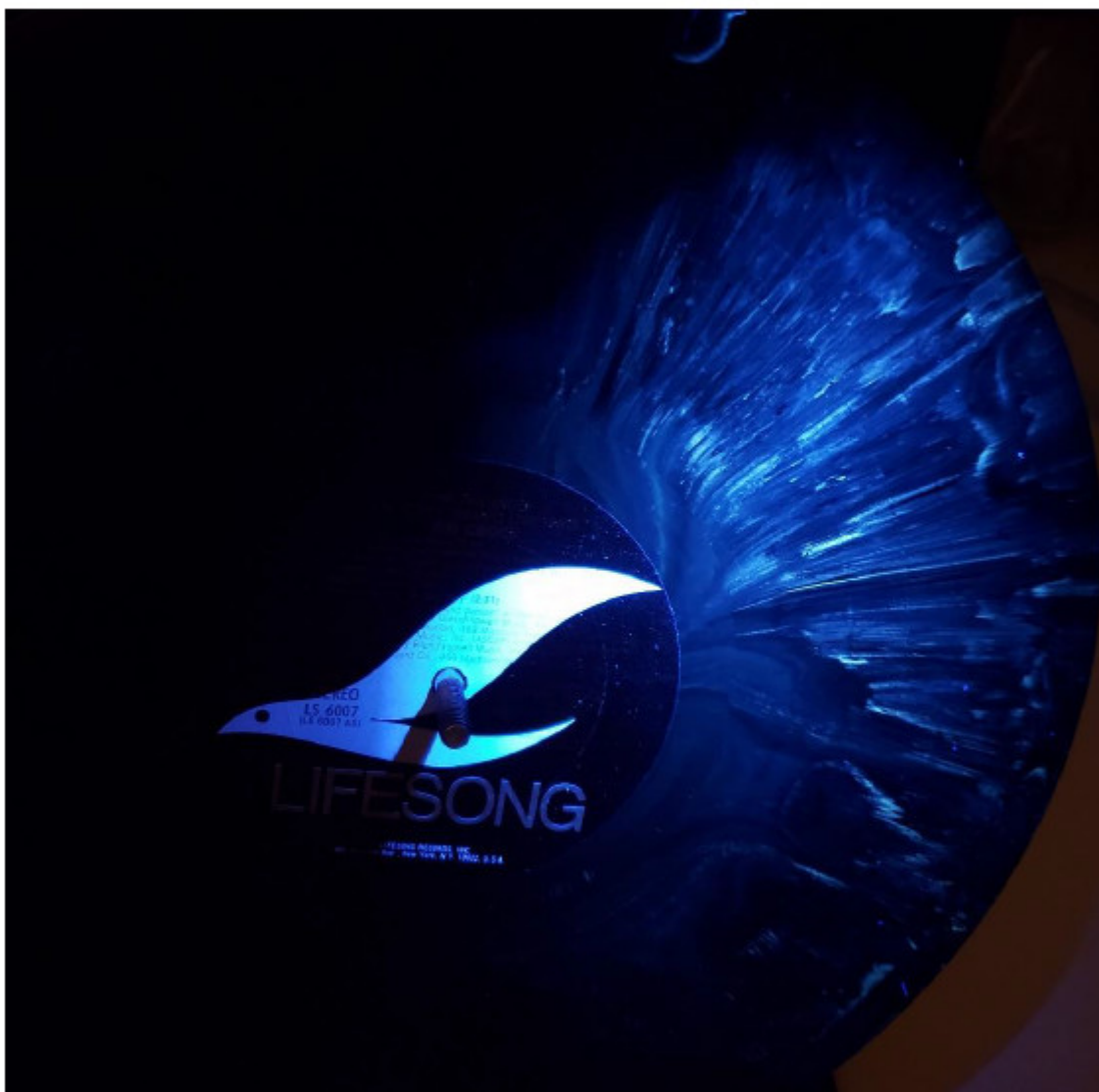
Figure 10 – Record Inspected UV Light – with Major Staining
