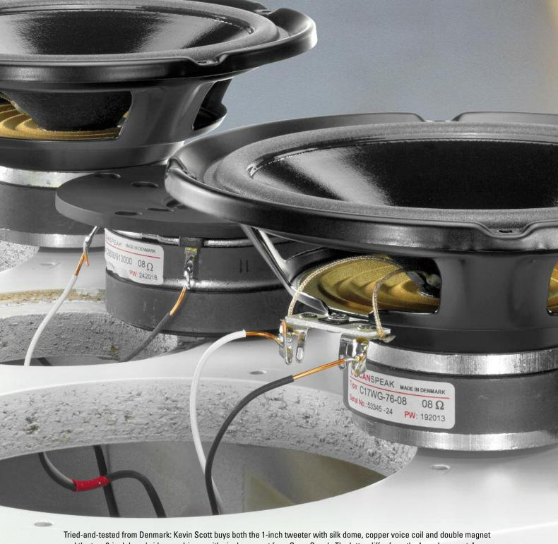
Tried-and-tested from Denmark: Kevin Scott buys both the 1-inch tweeter with silk dome, copper voice coil and double magnet and the two 6-inch bass/midrange drivers with single magnet from Scan-Speak. The latter differ from the "usual suspects" mainly by the shallow curvilinear diaphragm and the narrow diameter copper voice coil
