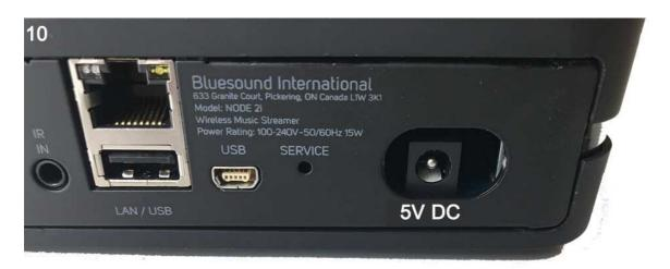
Re fit the back panel and plug in your Fidelity Audio PSU via the dc socket.
