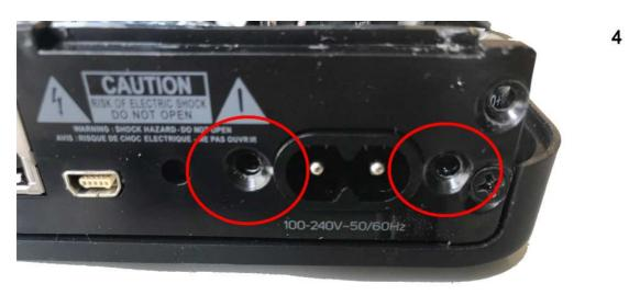
Remove two silver screws from ac input
