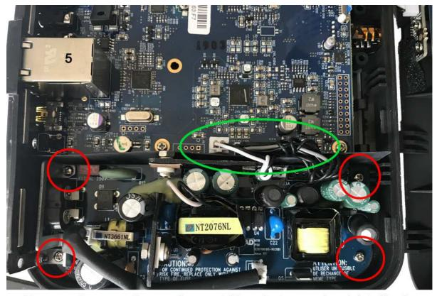
Remove 4 screws from pcb + metal bracket around ac inlet. Unplug the two connectors from the Bluesound pcb.
