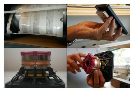
Below the ironless midrange/tweeter, above left the ribbon without chassis, above right the finished ribbon tweeter.
