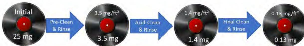
**Figure 42 - Record NVR Following Precision Aqueous Cleaning Process**
