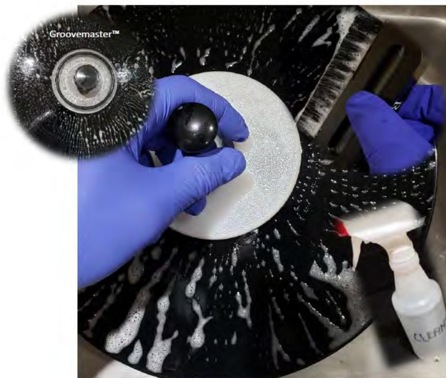
Figure 17 - Step 4: Pre-Clean with CLEANER Solution & Brush
