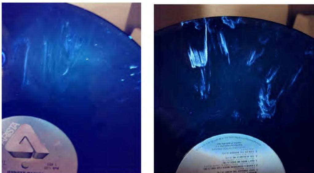
**Figure 9 - One Record Inspected UV Light - Heavily Soiled with Staining**
