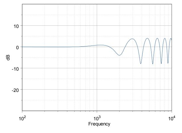
Figure 2 - Filter response for delay = .6 ms, + 4 dB stimulus.
