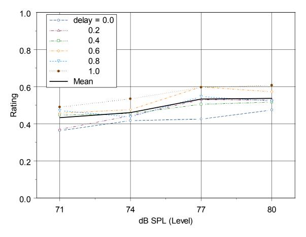
Figure 5 - Ratings versus playback level for +6 dB linear distortion with delay as a parameter. These ratings are significant at .005.
