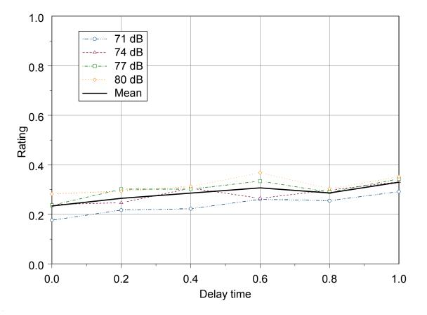
Figure 6 - Ratings versus delay for +4 dB linear distortion with playback level as a parameter.
