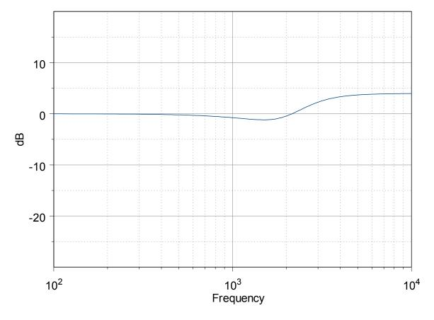
Figure 1 - Filter response for zero delay + 4 dB stimulus
