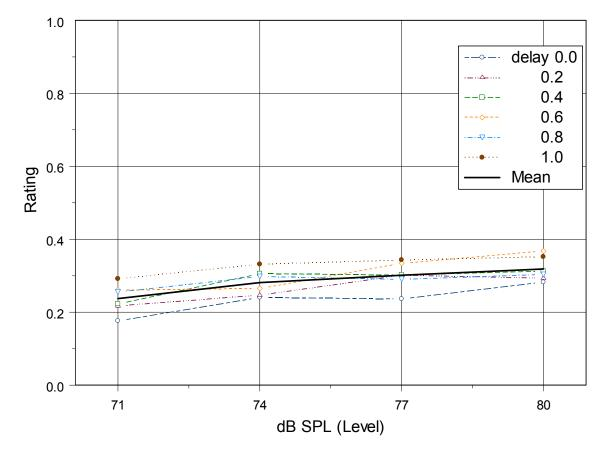
Figure 4 - Ratings versus playback level for +4 dB linear distortion with delay as a parameter. These data are significant at .05.
