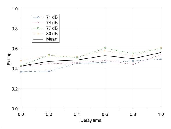
Figure 7 - Ratings versus delay for +4 dB linear distortion with playback level as a parameter.
